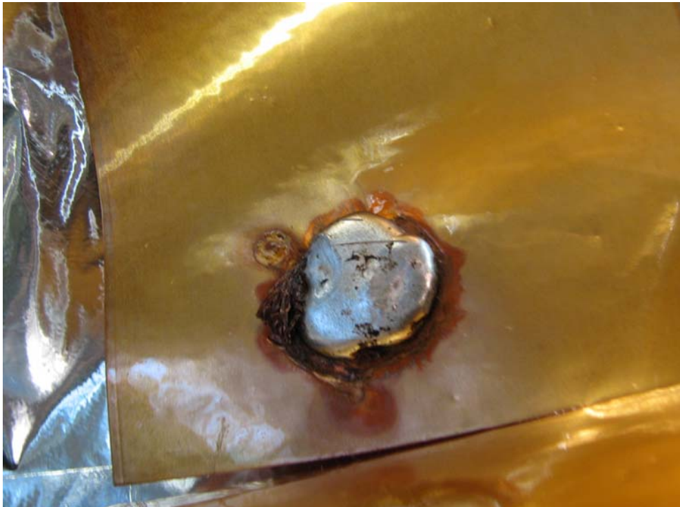
Discoloration at Tap Layer Interface, H1 FIGURE 8
