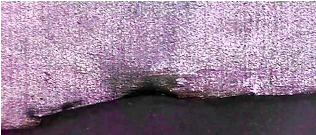
H1, BURNT FOIL EDGE x35 MAGNIFICATION FIGURE 11
