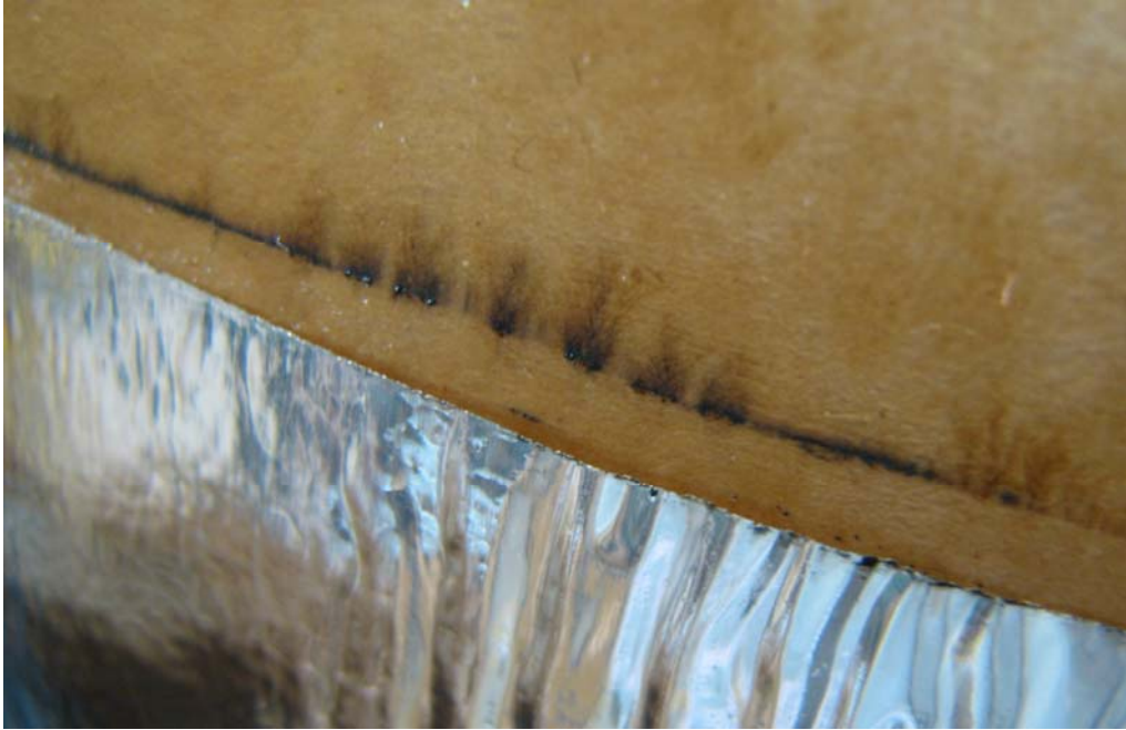
Discoloration at Foils Edge, H1 FIGURE 7
