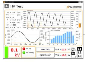
While performing tests, all necessary values like test voltage, PD-level, frequency, dissipation factor as well as a PD-pattern are shown in a single screen.
